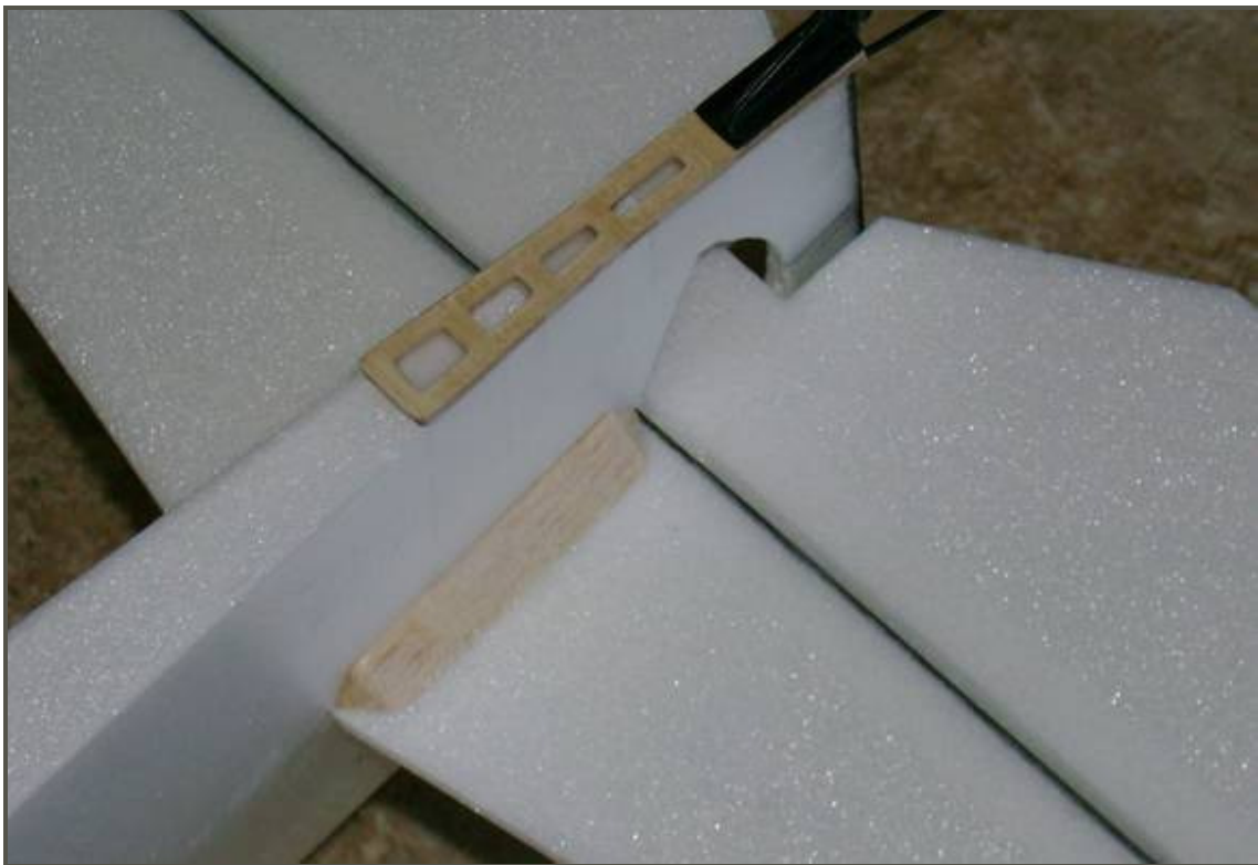
Figure 16 - Horizontal Stabilizer Balsa Doubler Detail
